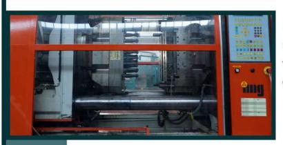
Maspi has several overmolding machines used for selected parts of furniture products or for projects in electrical and industrial fields.
