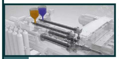
Restylon is the co-injection plastic transformation process that combines two compatible polymeric materials, using at least 30 percent recycled plastic without compromising the aesthetic end of the article.
